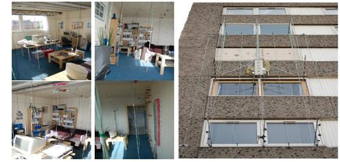
DFT1: A realistic modern day compartment scenario fire, comprehensively instrumented to enable thorough characterisation of compartment fire. External heat flux distribution to façade in good agreement with Law Model but not conservative as expected for design.
