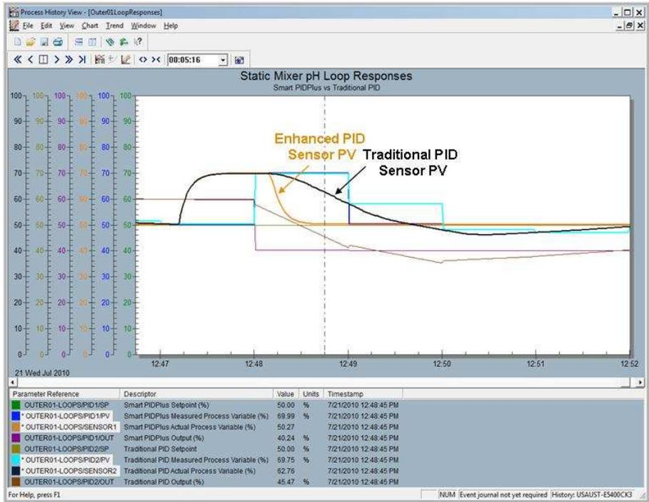
Figure 15. For a Wireless pH Loop Load Upset, the Enhanced PID Makes a Single Reagent Correction whereas the Traditional PID Slowly Makes a Series of Corrections
