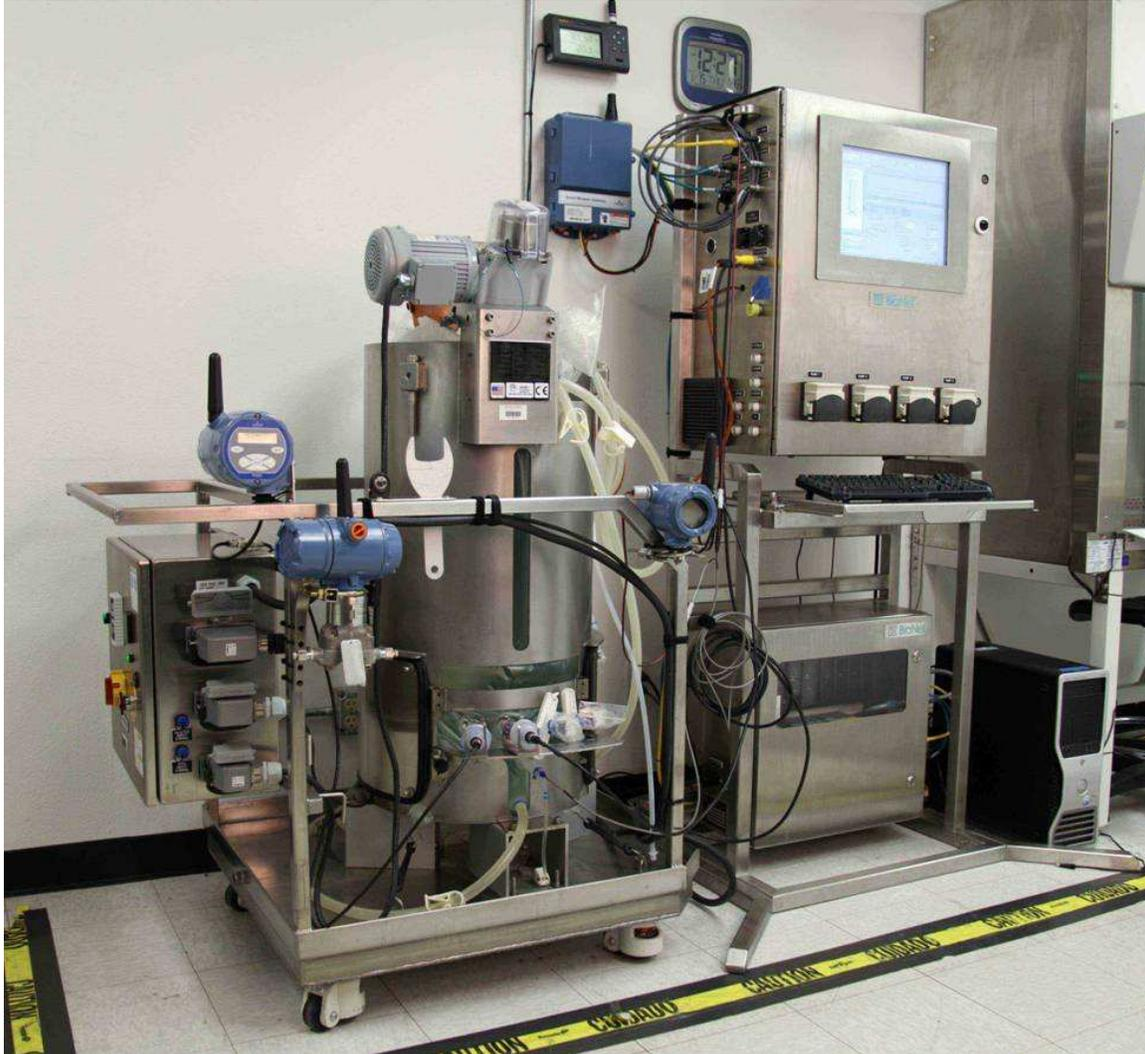
Figure 11. Wireless pH Transmitter on a Single Use Bioreactor
