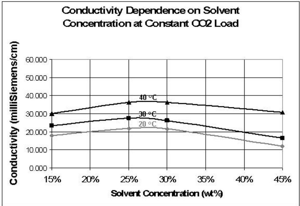
Figure 7. Conductivity for Inferential Measurement of Solvent Concentration had Poor Process Sensitivity and Reversal of Process Action Sign
