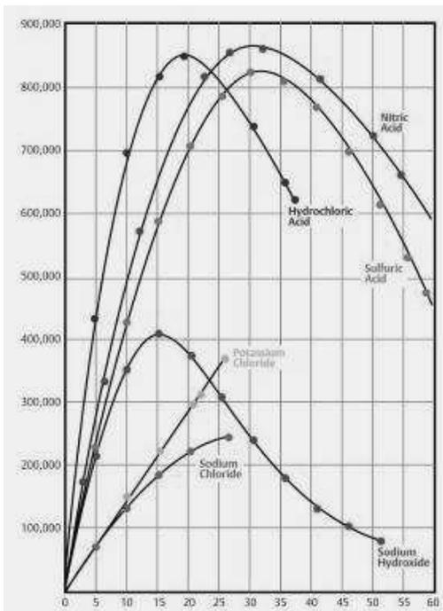
Figure 4. Conductivity as an inferential measurement of concentration can be used if the operating range can be verified to be always on one side of the peak.
