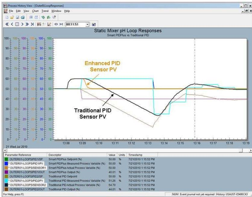
Figure 17. For a Wireless pH Loop, the Enhanced PID Rides out a Communication Failure or Broken Electrode whereas the Traditional PID Ramps to its Output Limit
