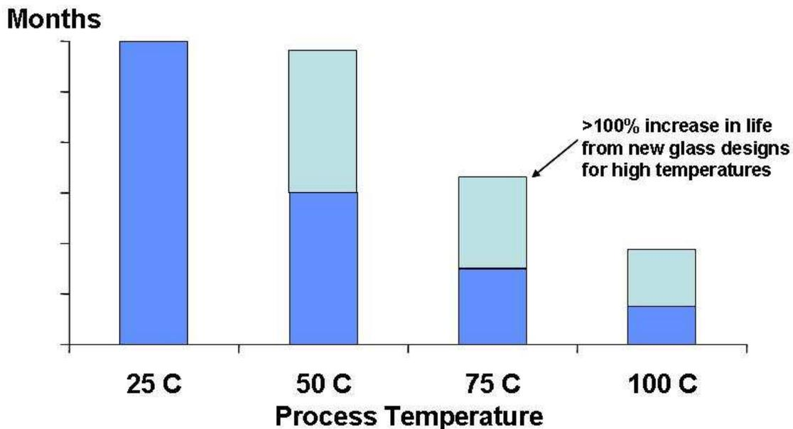
Figure 1. The life expectancy that decreases with temperature can be doubled by the use of new high temperature glass formulations.
