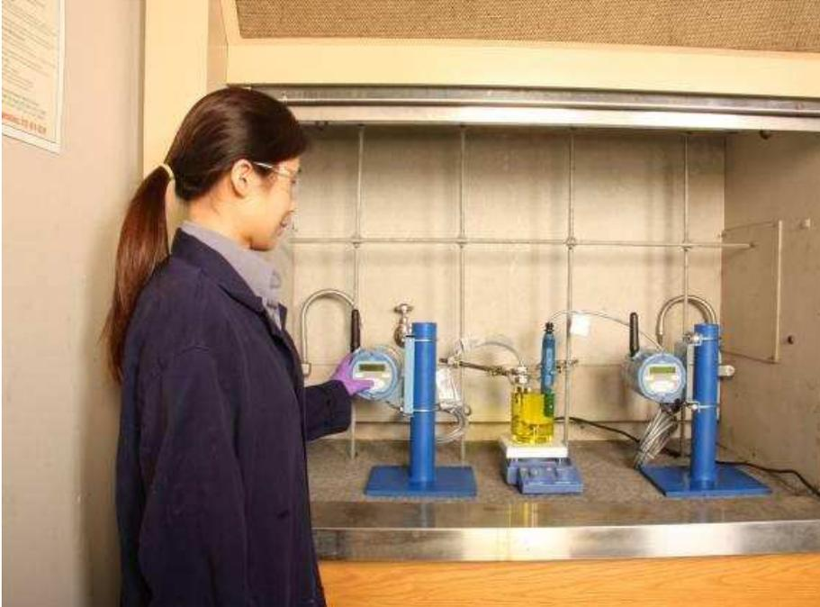
Figure 6. Wireless Test Setup of Conductivity and pH Transmitters for CO<sub>2</sub> Recovery
