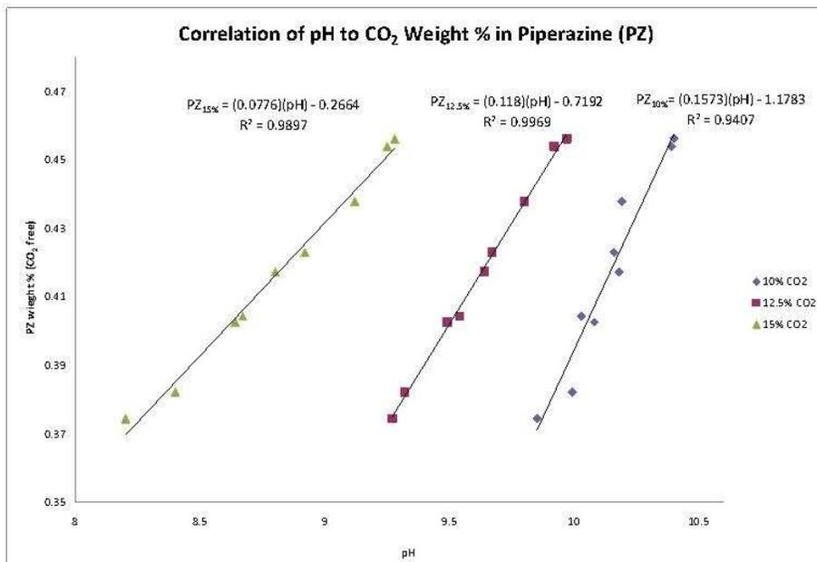
Figure 10. pH can be an Inferential Measurement of Piperazine (PZ) Solvent Concentration if the Solution pH is Compensated for CO<sub>2</sub> Loading and Temperature
