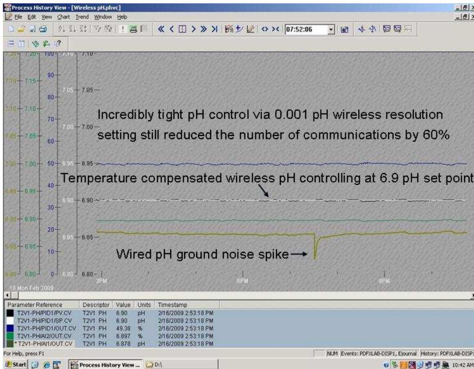
Figure 12. Wireless pH Transmitters Do Not Exhibit Spikes Seen in Wired Transmitters
