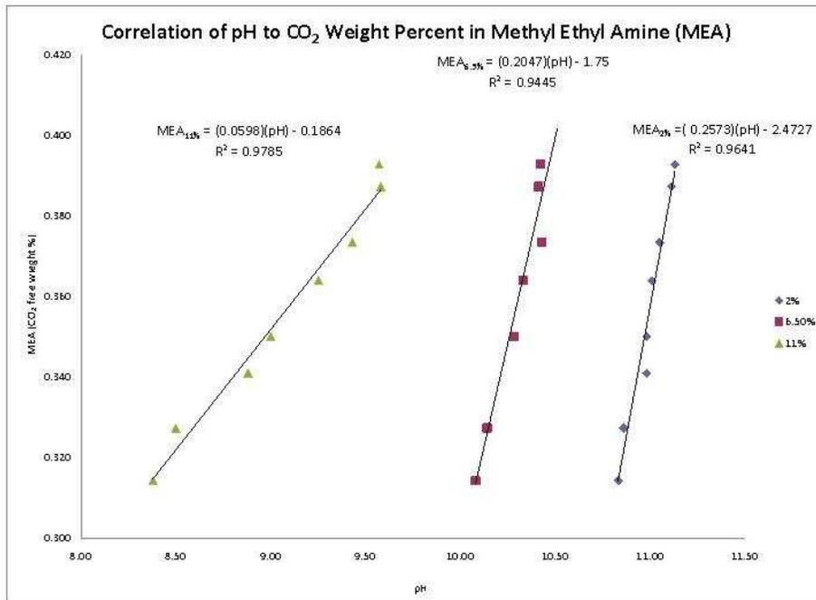
Figure 9. pH can be an Inferential Measurement of Methyl Ethyl Amine (MEA) Solvent Concentration if the Solution pH is Compensated for CO<sub>2</sub> Loading and Temperature
