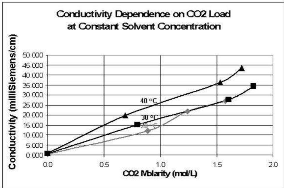
Figure 8. Conductivity for Inferential Measurement of CO<sub>2</sub> Loading Showed Promise if Proper Temperature Compensation is Developed and Automated.
