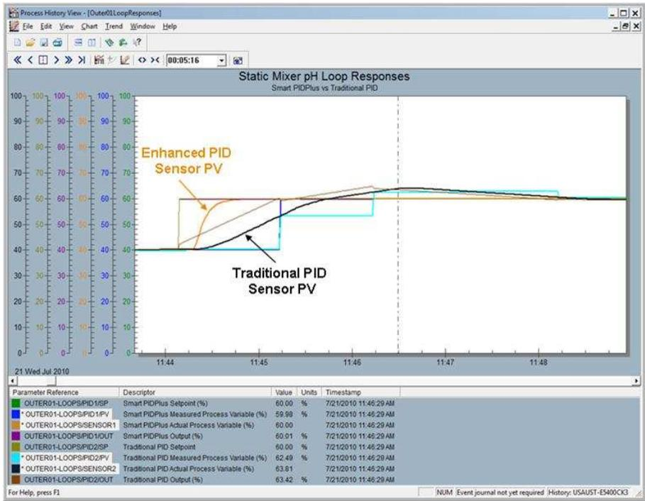
Figure 16. For a Wireless pH Loop Setpoint Change, the Enhanced PID Makes a Single Reagent Correction whereas the Traditional PID Slowly Makes a Series of Corrections
