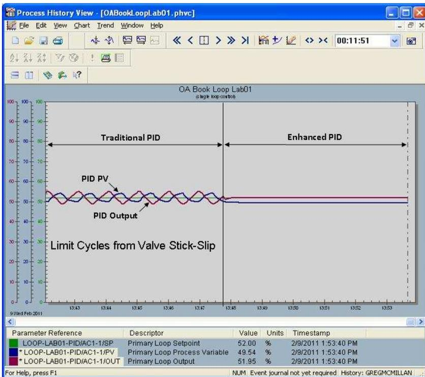
Figure 18. The Enabling of the Enhanced PID option for Wireless Control Eliminates Limit Cycles from Valve Stick-Slip and Backlash
