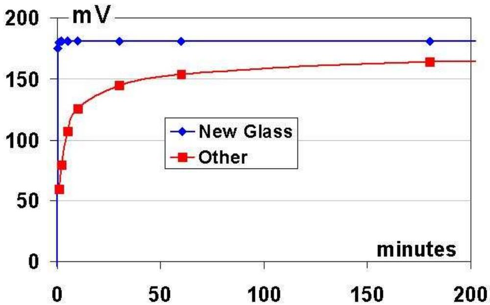
Figure 2. The onset of premature aging of the glass that greatly increases the response time can be delayed by the use of new high temperature glass formulations
